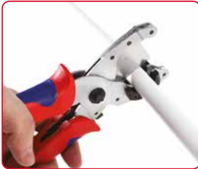
1. Cut the pipe at a 90° angle.
