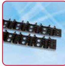
Maincor Clamp Track is designed to secure 16mm pipe. It has a self adhesive backing for ease of installation. Allow 1m for every m<sup>2</sup> of floor area.
