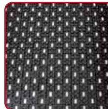
Maincor Pipe Positioning Panels are used for securing 16mm pipe within screeded floors. The castellated panels allow for the pipe to be secured at 50 - 300mm centres. Insulation is not included. The panels are to be overlapped. Each board covers an active area of (0.8m x 1.4m) 1.12m<sup>2</sup>
