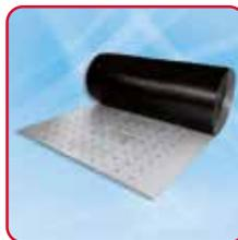
Maincor Screed Foil is designed to be placed directly on top of the floor grade insulation, providing a greater level of reflective insulation. Supplied in 60m x 1.25m x 4mm rolls. Thermal resistance = 0.081m<sup>2</sup>K/W.
