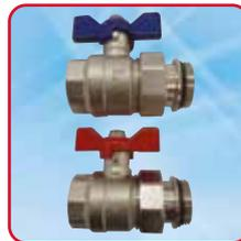
Maincor Straight Ball Valves are used to provide isolation of the flow and return pipework connected onto the Radiator Manifolds. This allows manifolds to be isolated both for filling the system, or draining down, without the risk of air ingress.
