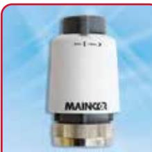
The manifolds are supplied with blue caps on the return manifold (bottom header) which isolate the return water. The blue caps can be removed to allow for either 24 or 240V electro-thermic heads to be fitted which open and close to control the flow of water around the heating circuits.
