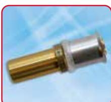
Press to Copper Compression Tails are used to connect MLCP fittings to standard copper compression fittings to enable simple system connection. Soldered fittings are not to be used with the press to copper tails since it's likely the internal O-ring will be damaged by the heat.
