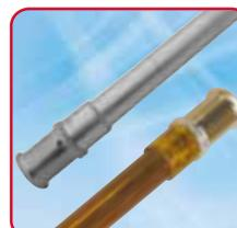
Use for making a press to press connection of MLCP and copper. The correct pressing jaws must be used for both the MLCP and copper connections. The fittings are not suitable for use with soldered fittings. The unplated version is also suitable for use with copper compression and pushfit fittings.
