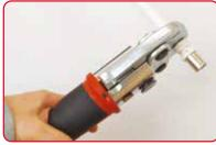
Insert the pipe into the fitting and 5. Using a standard Maincor 'U' profile 6. Joint Complete. press jaw and press tool, make the connection.
