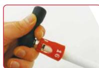
2. Bevel the cut end of the pipe.
