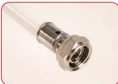
4. Fitting positioned on the end of the pipe - note there is no pipe in the viewing window.
