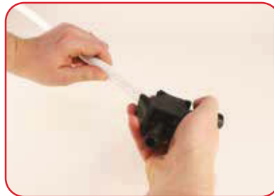
2. Bevel the cut end of the pipe.
