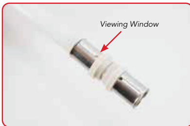
4. Insert the pipe into the fitting and check that the pipe is visible in each of the 3 viewing windows.
