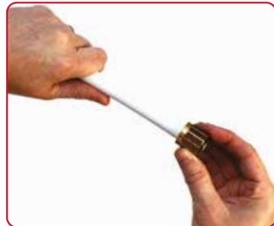
6. Fitting is now ready to tighten onto threads with straight BSP connections. Tighten the nut by hand until you meet resistance then use professional wrenches to further tighten the nut.
