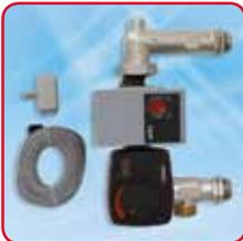
The Maincor Weather Compensated Control Pack modulates the flow temperature to the system requirements depending on outdoor weather conditions.
