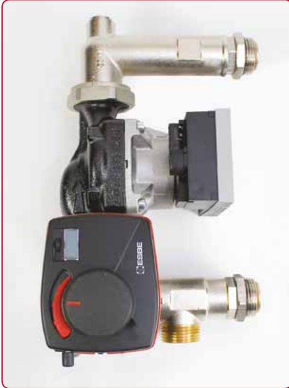
The Weather Compensated Control Pack WC250 is a pre-assembled water blending and pumping unit which is designed to be connected, via ball valves, to the UFH manifold. The unit modulates the flow temperature to the system requirements depending on outdoor weather conditions.
