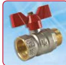
Maincor Straight Ball Valves are used to provide isolation of the flow and return pipework connected onto the Underfloor Heating Manifolds. This allows manifolds to be isolated both for filling the system, or draining down, without the risk of air ingress.
