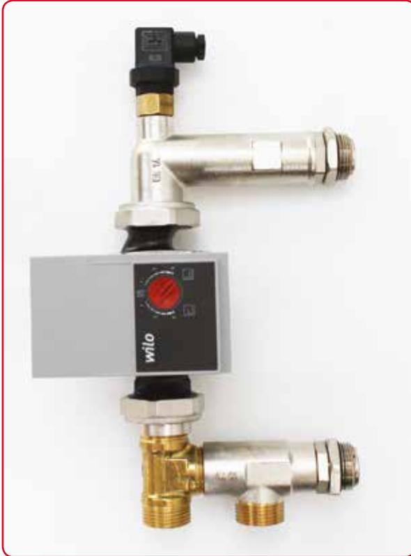
The Maincor Heat Pump pack HP250 is for use in applications when water blending controls are not required. Ideal for use with heat pumps installations or other renewable technologies that deliver heating water at a lower temperature than conventional gas boilers. The pack is suitable for use with floor areas of up to 250m<sup>2</sup> or a maximum output of 20kW.
