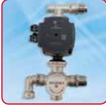
The Maincor Control Pack is a preassembled unit designed to be easily fixed (via the ball valves) to the UFH Manifold. The unit will blend the primary hot water with the return water from the UFH to the temperature that is determined by the control valve. An A rated pump
