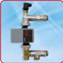
The Maincor Heat Pump pack is for use when water blending controls are not required. The unit is pre-assembled and is designed to be fitted on to either side of the manifold. A high limit shut off is included and pre-set to 60°C.
