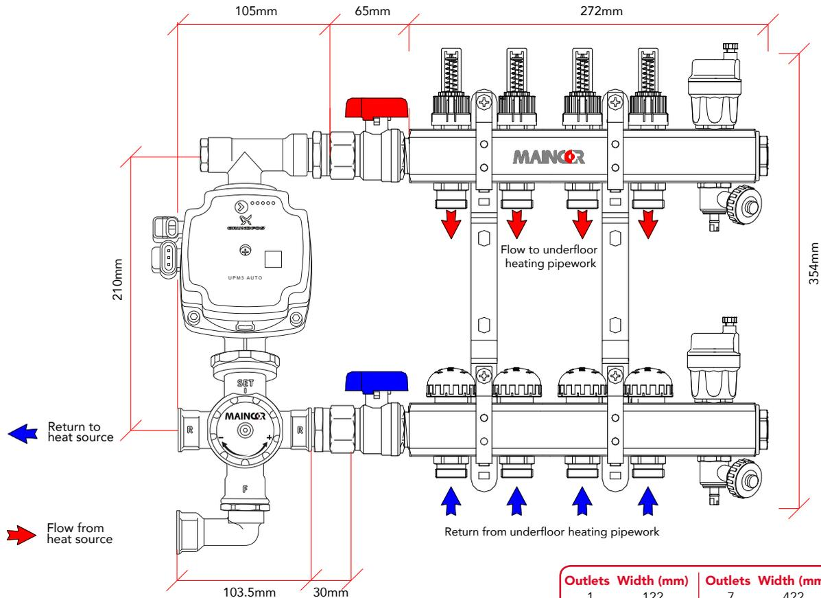
Primary pipework can be fed into the Control Pack from the side (as per the illustration) or from below by moving the position of the 90°elbow supplied with the kit.
