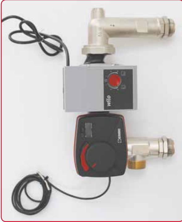
The Control Pack CP250 is a pre-assembled water blending and pumping unit which is designed to be connected, via ball valves, to the UFH manifold. The pack is suitable for use with floor areas of up to 250m<sup>2</sup> or a maximum output of 20kW. It is good practice to fit a 2 port motorised zone valve on the primary flow to manifold and Maincor will usually supply one. We recommend fitting an automatic bypass (supplied by others) on the primary flow prior to the 2 port motorised zone valve.
