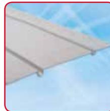
Maincor Heat Emission Plates are for use in timber suspended floors where the joists are at 400mm centres, or in floating floor applications. The plates are 390mm wide x 1m in length. Allow 2.2 plates per m<sup>2</sup> of floor area 16mm pipe at 200mm centres. Varying pipe sizes and centres available on request.
