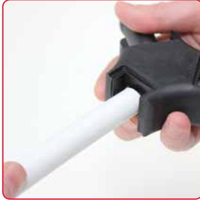
2. Bevel the cut end of the pipe
