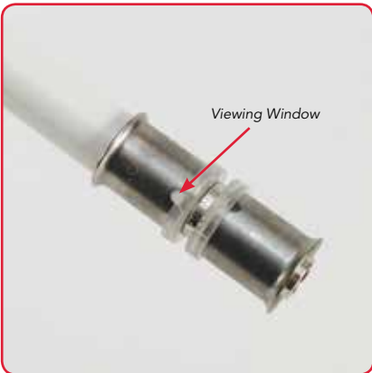
4. Insert the pipe into the fitting and check the pipe is visible in the viewing windows
