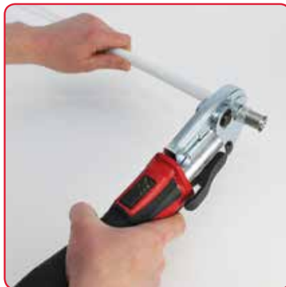
5. Using a Maincor Pressing Tool or Mini Pressing Tool, make the connection
