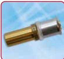
Press to Copper Tails are used to connect MLCP fittings to standard copper compression fittings to enable simple system connection. Soldered fittings are not to be used with the press to copper tails since it's likely the internal O-ring will be damaged by the heat.
