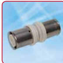
Maincor Straight Press Couplers / Reducers are used where straight lengths in excess of 5m are required. By utilising the straight press fitting, multiple 5m lengths can be coupled together, giving the desired installation length.
