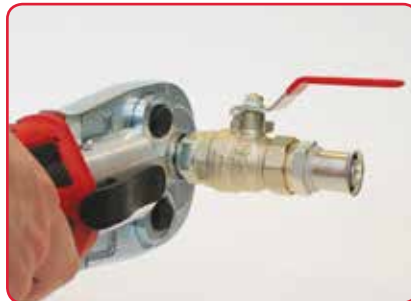
5. Using a Maincor Pressing Tool or Mini Pressing Tool, make the connection
