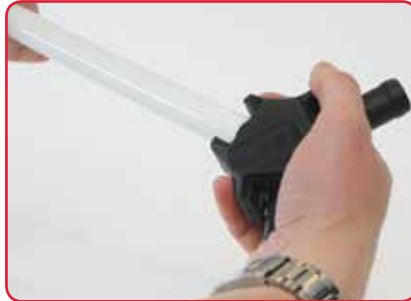
2. Bevel the cut end of the pipe
