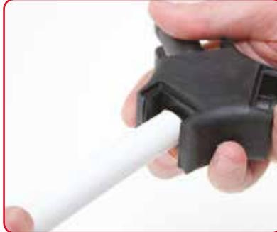
2. Bevel the cut end of the pipe.
